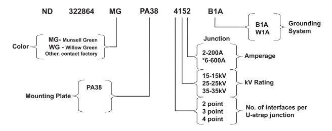
\*This cabinet will accommodate 15-35kV, 200 & 600Amp junctions with U-straps. It will accommodate 200Amp taps off the 600Amp deadbreak junction. It will also accommodate Cooper 35kV 200/600Amp loadbreak junctions.
